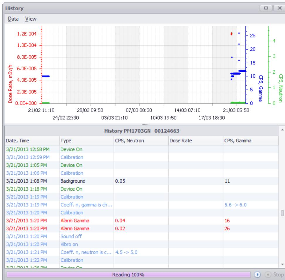
At the top of the window there is the area for graphical displaying of the measurement. Below there are measurement data represented in tabular style. The first column shows the date and time of measurement in chronological order; 2 - the type of event; 3 - CPS, Neutron; 4 - Dose Rate; 5 - CPS, Gamma.
