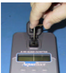
Photo 3. Adjusting the value on the secondary standard by turning the attenuation screw.
