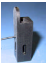
Photo 1. Loosening the locking setscrew on the backside of the adjustable secondary standard
