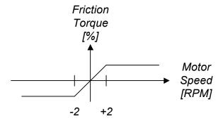
When the rotational speed reference reaches +/- 2 RPM, the output is a fixed torque, representing a kinetic friction torque component. A static friction component is not included.
