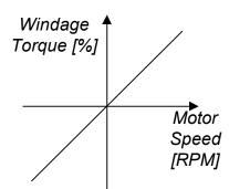
The inertia and losses torque return parameter is computed as the sum of inertia torque, friction torque and windage torque.
