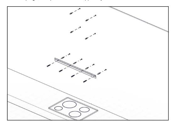
4- Hang the hood, aligning the wall support to the hook in the rear of the hood.
