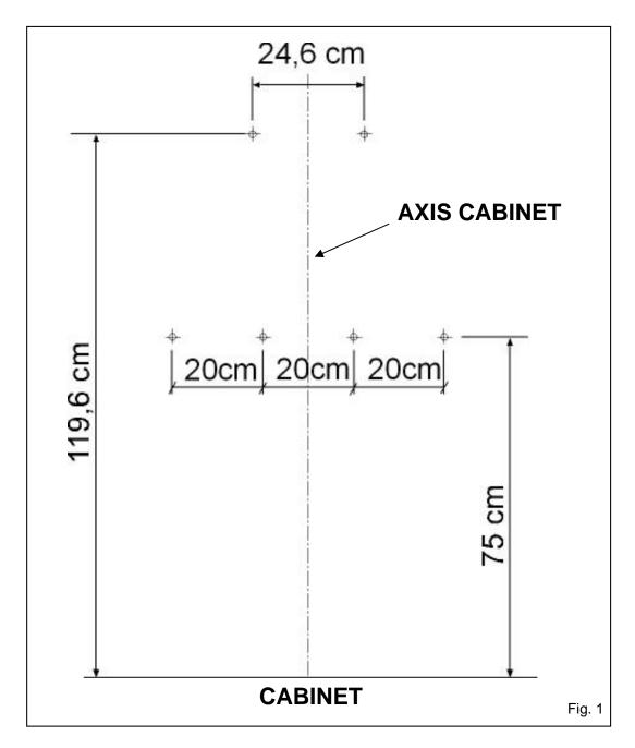
Advertise: This measures are the recommended for the installation, therefore for the CURVE C version as for the CURVE L version.
