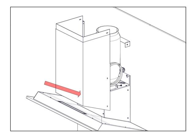
9- Screw the external part of the decoratives flues at the body of the hood, and push up the internal flue till align the holes in with the others in the decorative flues's mounting bracket. It must cover totally the flexible flue. Then, screw the upper decorative flue.
