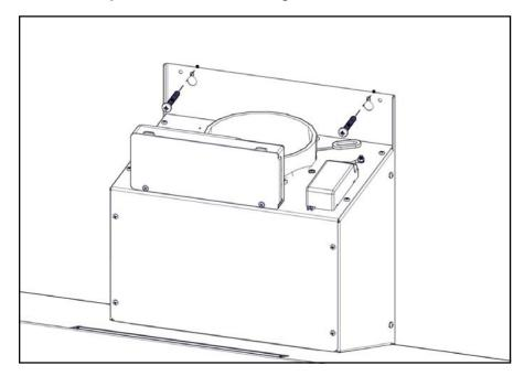
6- Intube the engine and the flue with the SEC tube, by following the tips of the User, Installation Manual. Fix the connections hermetically with the flanges.
