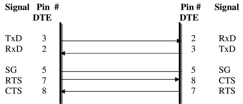
For loop back test, you can connect TxD(pin 3) to RxD(pin 2) and RTS(7) to CTS(8).
