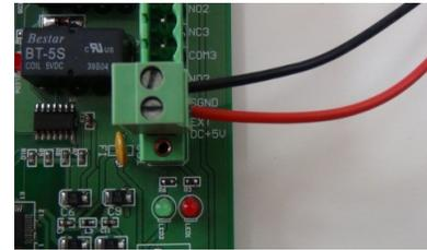
Attach the **black** cord to the **SGND** and the **red** cord to the **EXT DC+5V.**, as well as the signals cords
