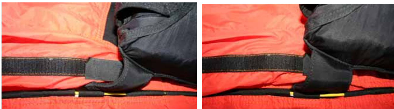
Photos showing the blank Velcro strip in position, with the rig pulled to the right for clarity.
