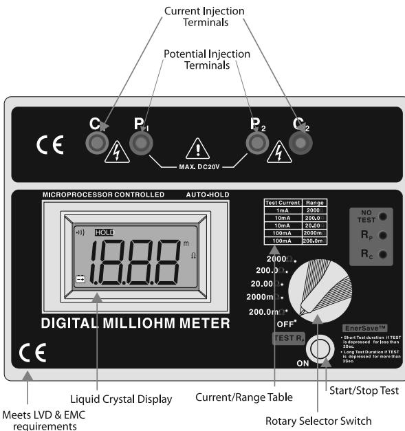
Always ensure the instrument is off before connecting any test leads.
