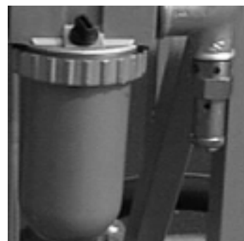
23 Safety valve for air maintenance unit
