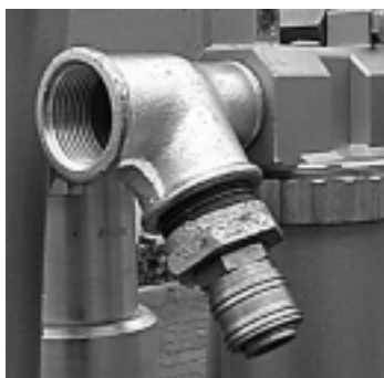
24 Air inlet for air maintenance unit
