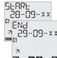
During normal operation, the possible execution of a holiday programme is signalled by the symbol in field (7) on the display.
