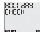
In case of HOLIDAY ONE DAY it is possible to scroll the programs using "C1" and "C2" keys. In case of HOLIDAY PERIOD the instrument shows the start day of the first holiday period, press "C2" to visualize the end of the period. At this point, pressing "OK" it is possible to access to options of modify, delete or next holiday period.
