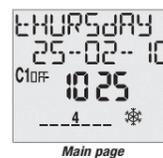
Note: if the instrument is not powered by the mains, instead of the day the following message will appear on the top row NO SUPPLY. In this condition backlighting is not active and the relay will remain off.
