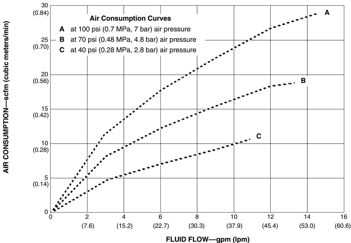
**To find Pump Air Consumption** (scfm or  $m^3/min$ ) at a specific fluid flow (gpm/lpm) and air pressure (psi/MPa/bar):
