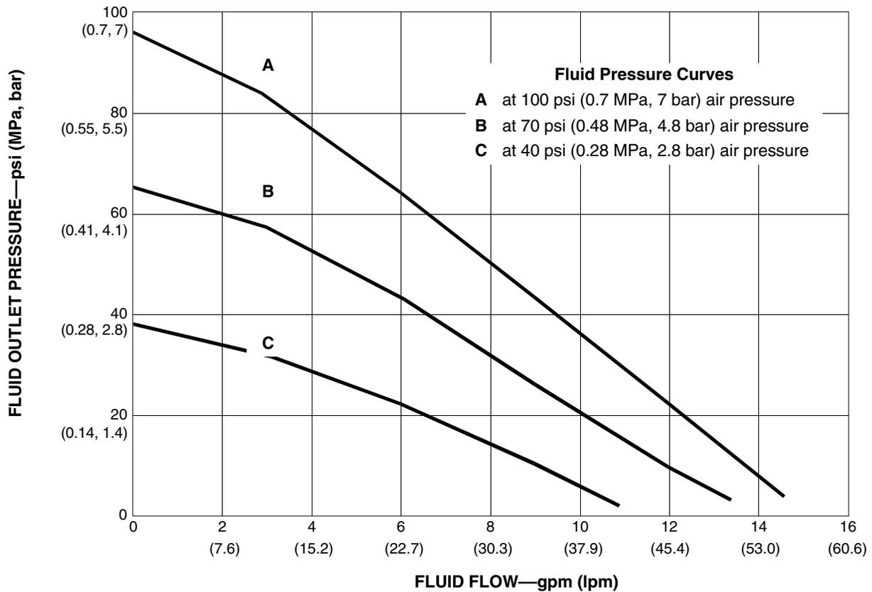
**To find Fluid Outlet Pressure (psi/MPa/bar) at a specific fluid flow (gpm/lpm) and operating air pressure (psi/MPa/bar):**
