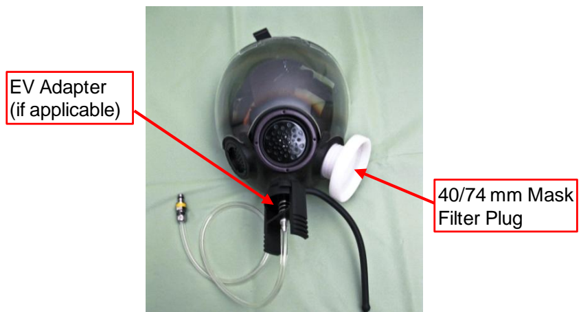
Example of Mask Filter Plug and EV Adapter installed on mask. This configuration may vary depending on the mask being tested.
