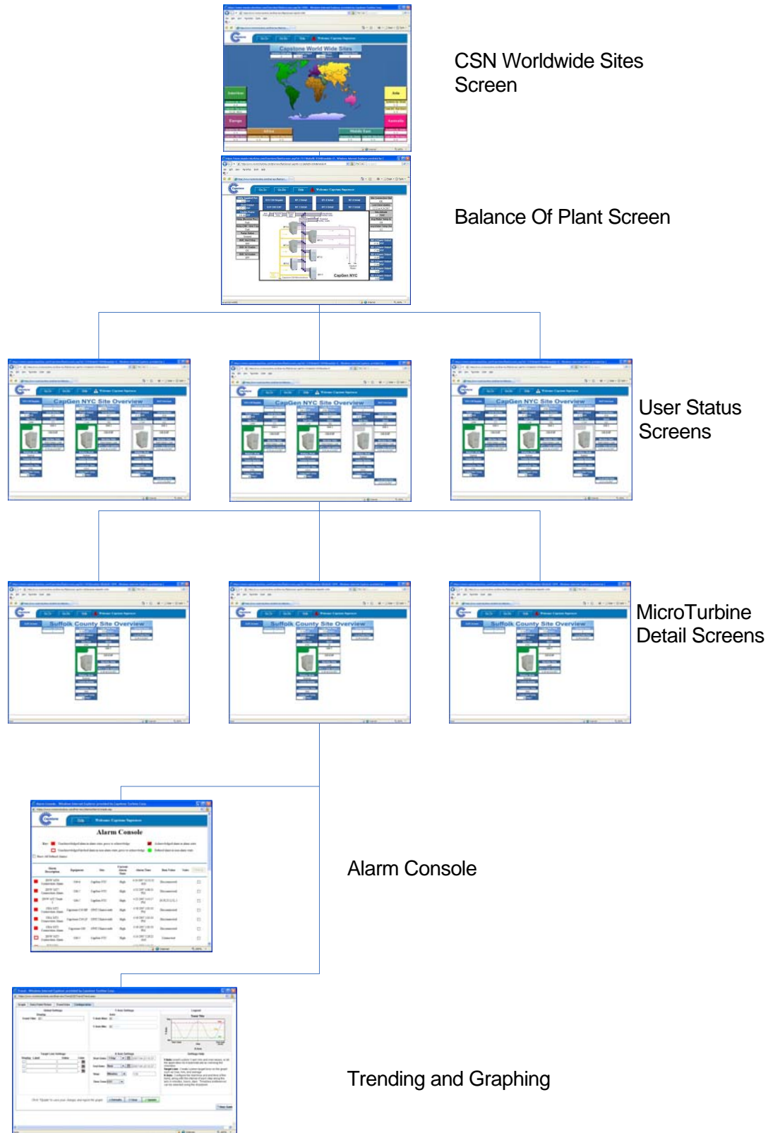
Figure 14. Any Number of MicroTurbines with Balance of Plant Monitoring
