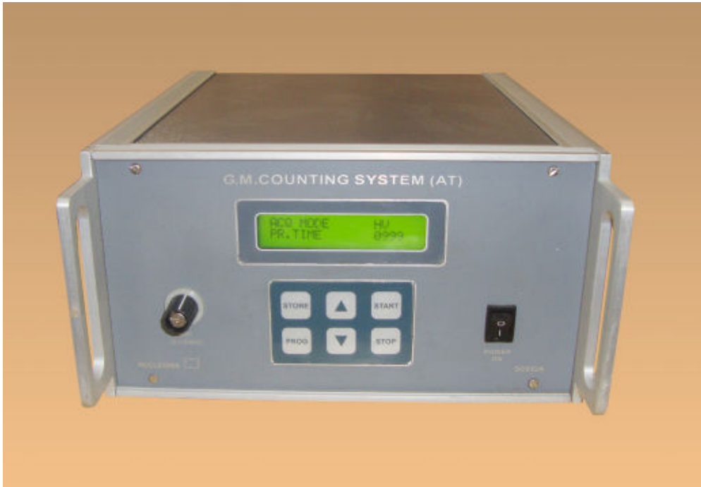
FRONT VIEW OF G.M COUNTING SYSTEM AT TYPE : (GC601A)
