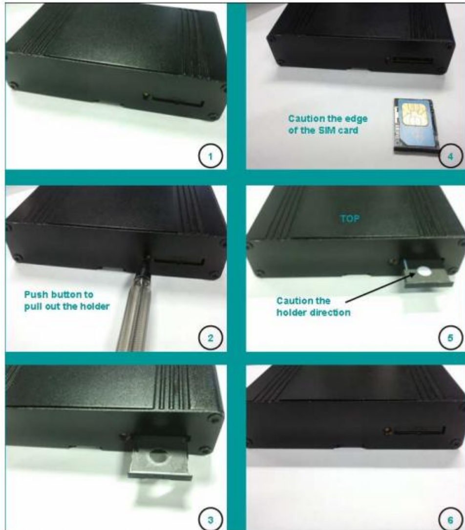
Figure 17: Installation of SIM card
