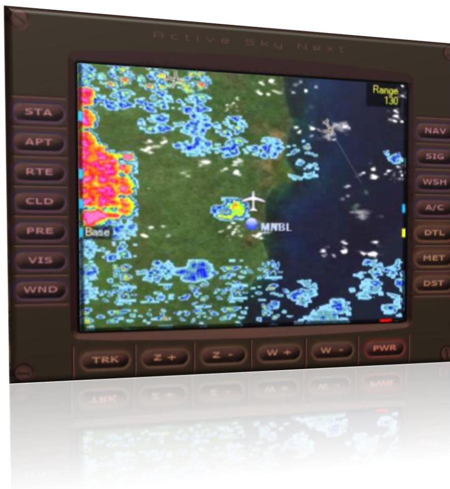
The buttons along the left and right side of the gauge provide overlay toggle control. Press the button once to turn an overlay on, and again to turn it off.
