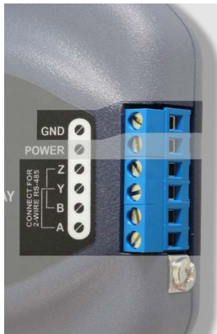
Figure 3: Terminal Block RS-485 Connections
