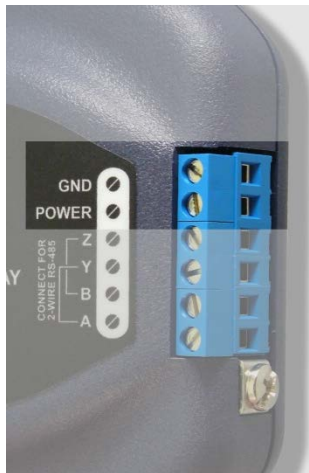
Figure 1: Terminal Block Power Supply Connections
