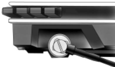
b. Connect the other end of the cable to the antenna connector on the transceiver:
