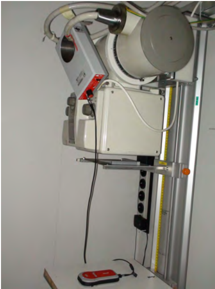
Figure 2.4 MAS-3 setup with Piranha as a trigger
