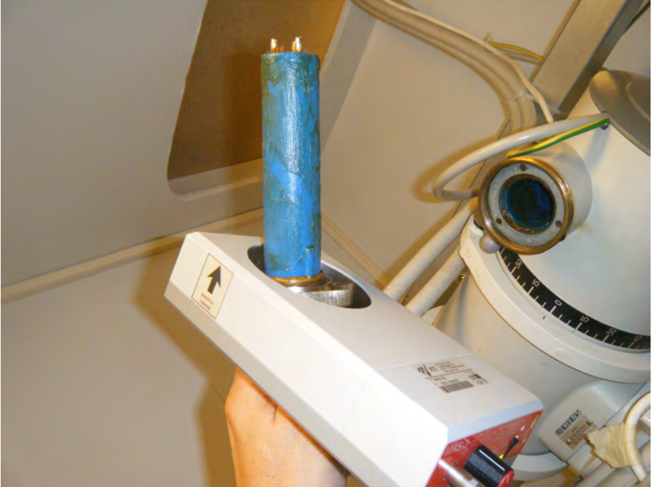
Figure 2.2 Anode cable disconnection and connection of MAS-3B Note the polarity of the probe. The arrow on the probe is pointing at the tube anode side.
