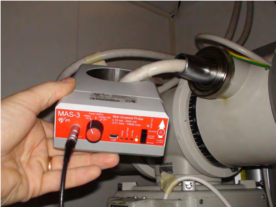
Connection of MAS-3B to a RAD tube
