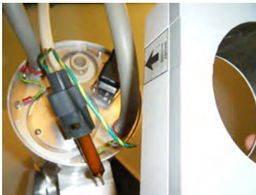
Connection of MAS-3B to a mammo tube
