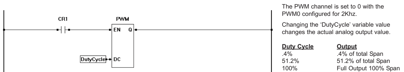
Figure 2.14 - Using PWM to Control Analog Outputs
