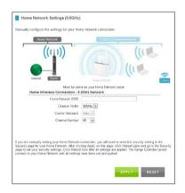
Channel Width: Wi-Fi operates in two separate channel widths, 20Hz and 40Hz. 40Hz allows for faster speeds. Each Channel Width will have a different selection of wireless channels to choose from. Select the channel width you wish to use for your network. This setting must match that of your Home Network for a successful connection.
