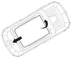
3. Replace the battery. Align the contacts of the battery with the corresponding connectors in the battery compartment.
