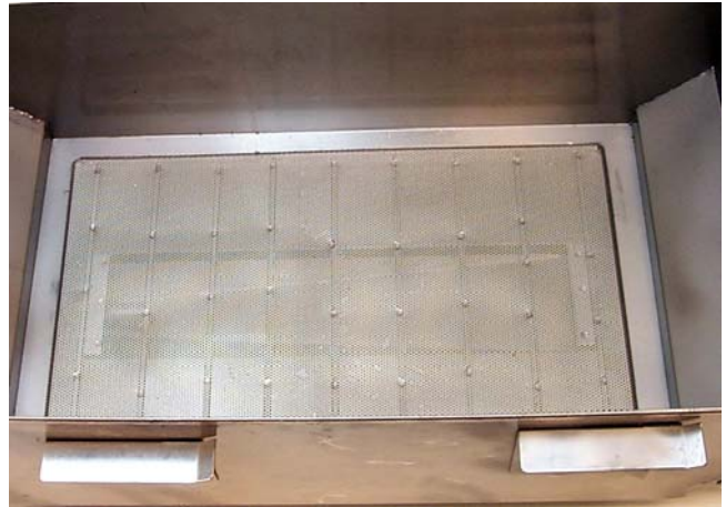
Support grid properly placed in filter pan.
