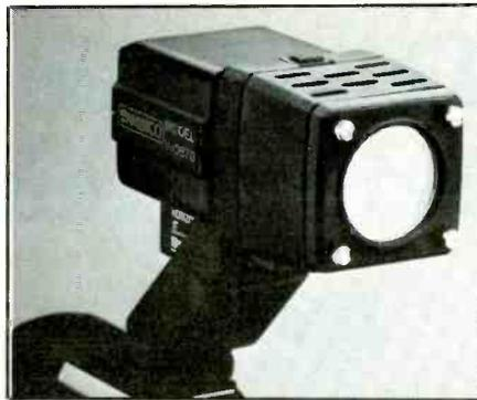
that spreads the light out evenly and eliminates glare. A lightweight Ni-Cd battery pack, which clips onto the light, provides power for up to 20 minutes. The battery pack can be recharged hundreds of times with the charger supplied with the light. The Powerlight mounts onto the light shoe of virtually any camcorder. \$129.95.
