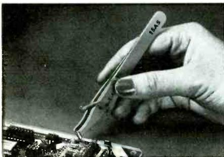
ducing muscle tension and thereby providing better muscle control for miniaturized work. The "E-Z" cutting device is available on 12 different cutting tweezers that have various blade configurations and sizes. The lever can be positioned to accommodate both right- and left-hand use.
