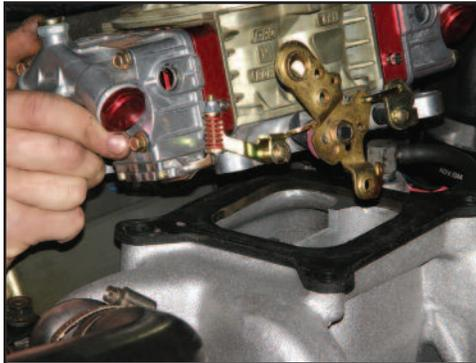
3. **Left** - Remove the carburetor following the vehicle manufacturer's guidelines.
