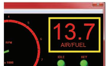
**Air Fuel Ratio:** This is displayed in two locations. It shows numerically the air to fuel ratio. The sample shows a 13.7 to 1 air to fuel ratio.
