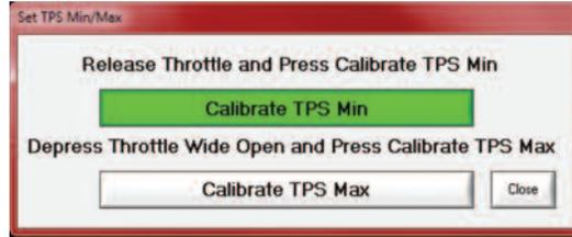
The TPS Calibration window will open. With the accelerator released and the throttle fully closed, press the "Calibrate TPS Min" button. Next depress the accelerator pedal fully to the floor and while fully held down, click the "Calibrate TPS Max" button.
