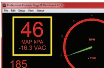
**MAP:** The MAP (Manifold Absolute Pressure) is displayed in both kPa and inches of vacuum or PSI. Zero inches of vacuum equals 100 kPa.
