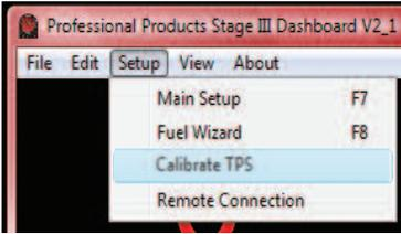
This next step is to Calibrate the Throttle Position Sensor (TPS). Click on "Setup" and select "Calibrate TPS."
