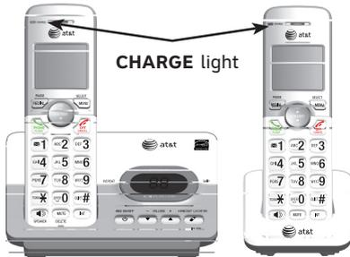
4. Charge the handset by placing it face up in the telephone base or charger. The **CHARGE** light is on when charging.
