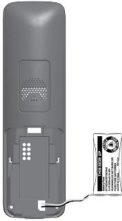
1. Plug the battery connector securely into the socket inside the handset battery compartment, matching the orientation of the engraved label.
