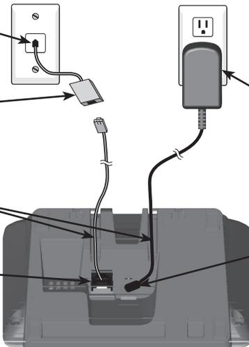
Plug the large end of the base power adapter into an electrical outlet not controlled by a wall switch.
