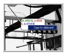
Right-click on a measurement bubble to copy values to the clipboard. This allows quick extraction of data for incorporation with other programs, or to add to reports etc.
