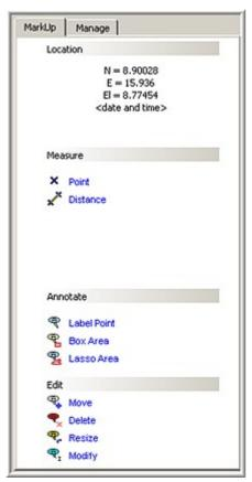
The *Mark Up* tab displays various tools to add and edit annotations and to make measurements in the scan bubble.
