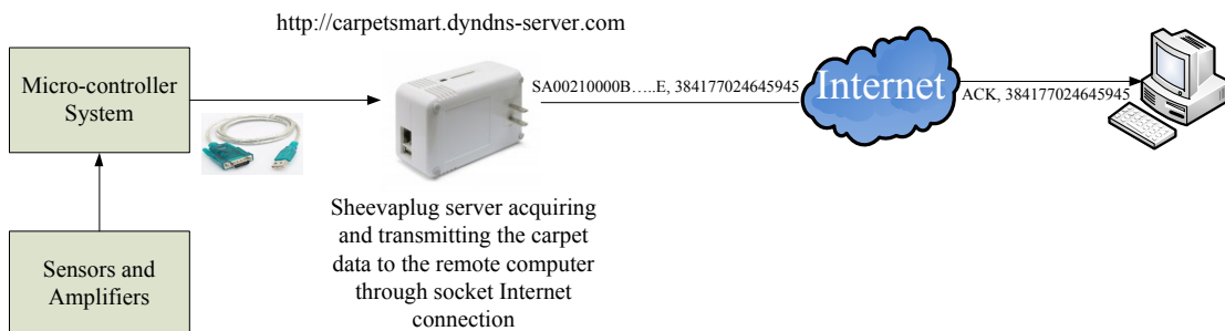
Figure 3-9: Block diagram describes the communication of carpet data from Sheevaplug server to the remote computer. The data is communicated over the socket connection between the server and the remote computer.
