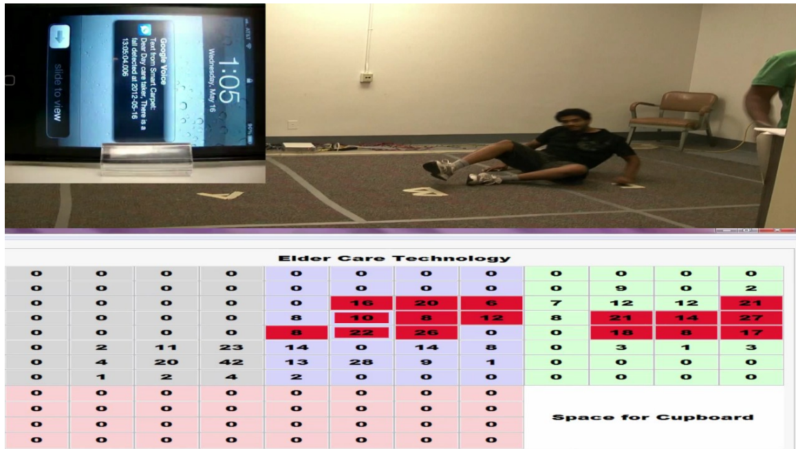
Figure 4-18: The Emergency notification in the form of text message is received on nurses' mobile after detecting the fall. The bottom part of this picture shows the way data is displayed on remote computer.
