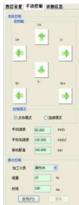
Fig.3-24 Control panel of auto feeding machine
