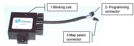
**Note**: *KLXCDI* pictured here is for North American 2006-2007 model years. 2009 and later have only one six pin connector on the unit. Australian models have flying leads with connectors.
