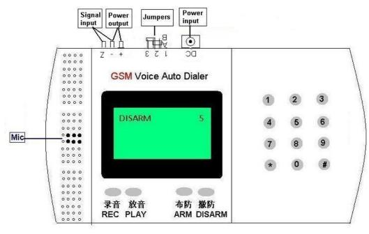
Mic: Microphone, face to the microphone when recording voice message
