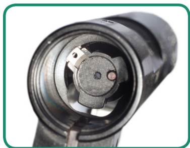
Fig. 8: extractor protrudes over the outside surface of the bolt
