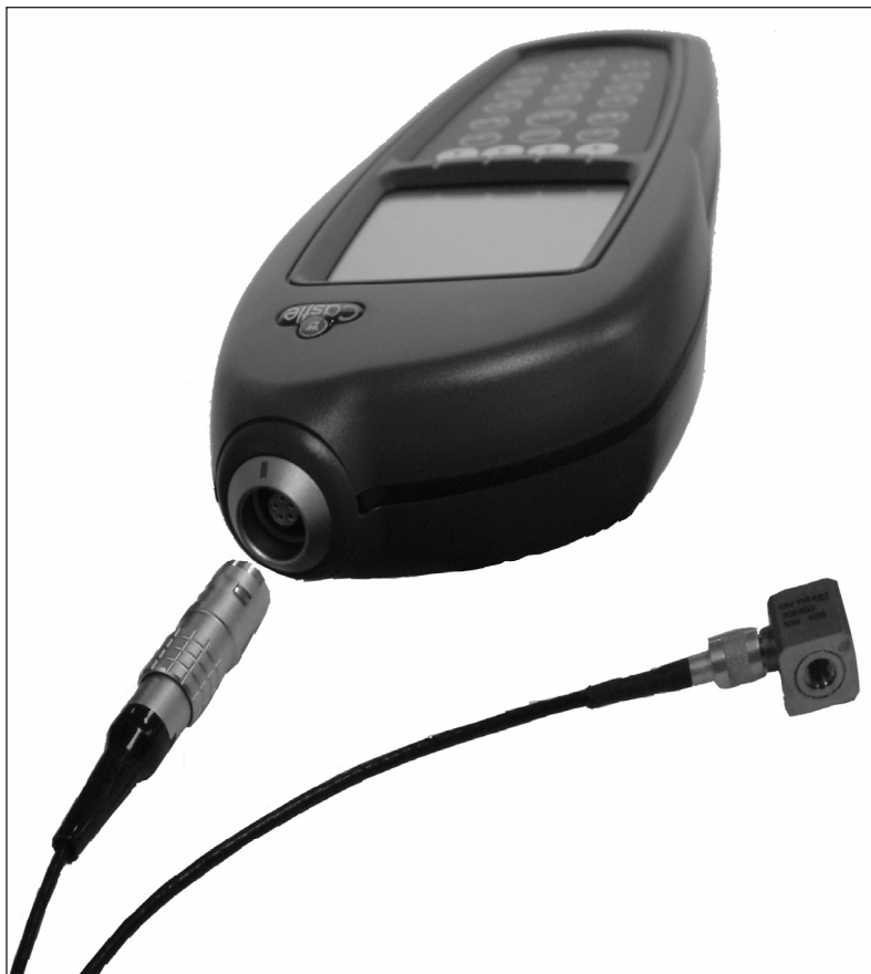
Figure 2 – Attaching Accelerometers to the Instrument
