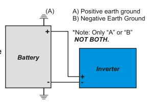
**CAUTION**: Before any connections are made to the Unit or System, be sure to disconnect the battery terminals. Always disconnect the grounded battery terminal first. When re-connecting, connect ungrounded terminal first, and grounded terminal last.
