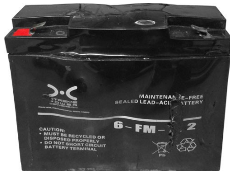
Temperature/Overcharged affected battery
