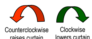
Diagram 8 For motor oriented with power cord to front, rotate hex wrench:
