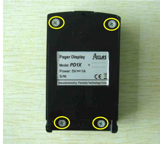
2. Use screwdriver to unscrew the four screws.
