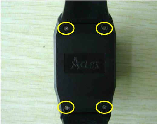
1. Use screwdriver to unscrew the four screws.
