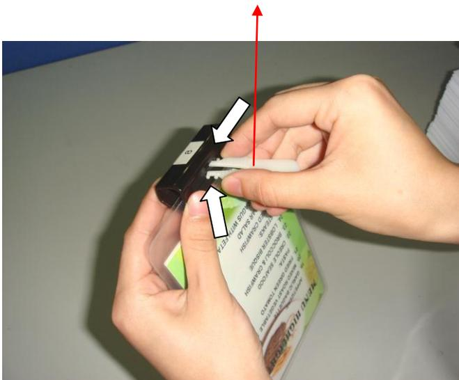
**Note: Press both sides of the bill clip towards the midst with two fingers, and then fix it into the clamp ring.**
