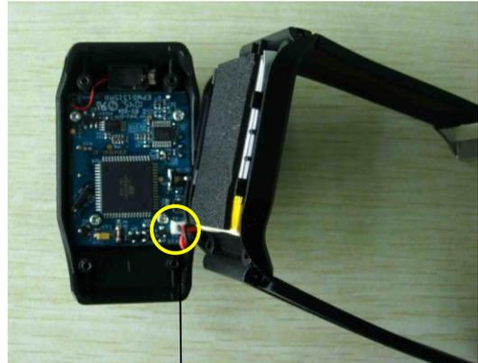
2. Open the cover, pull and plug the battery connection cables. Then reassemble the receiver in reverse order.
