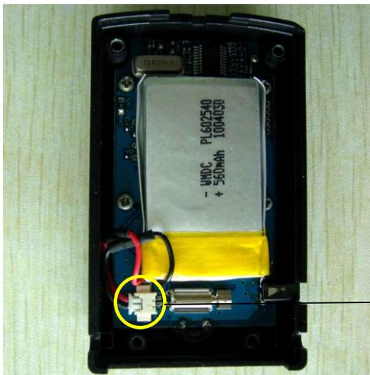
3. Open the cover, pull and plug the battery connection cables. Then reassemble the receiver in reverse order.
