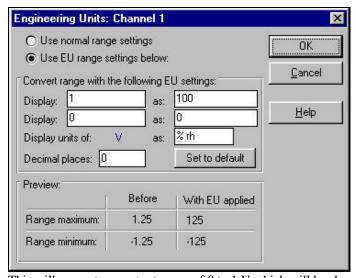
This will generate an output range of 0 to 1 V which will be shown as 0 to 100% rh.
