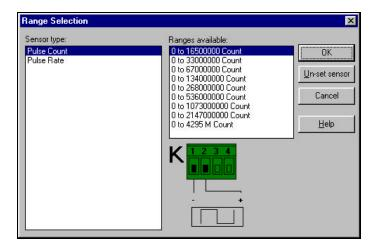
3. Select **Pulse Rate** from the **Sensor type** list. The available ranges for this sensor type will be shown, together with the wiring diagram:
