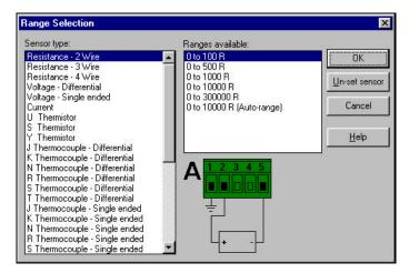
3. Select **Voltage - Differential** from the **Sensor type** list. The available ranges for this sensor type will be shown, together with the wiring diagram:
