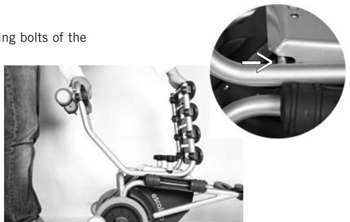
Fix the C-part tightly to the climbing frame with the two tightening knobs ❷.
