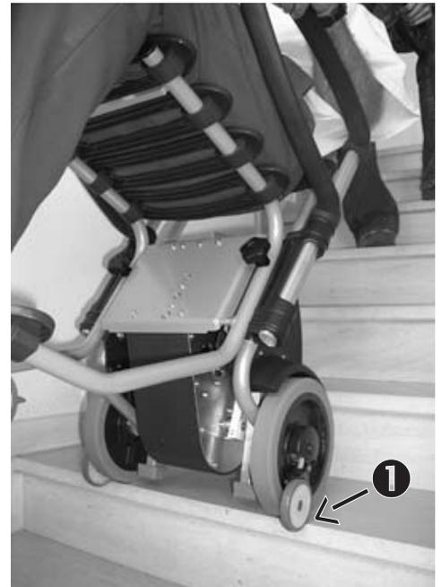
The sensitive rolls ❷ of the safety brakes keep the **escalino** from rolling over the edge.
