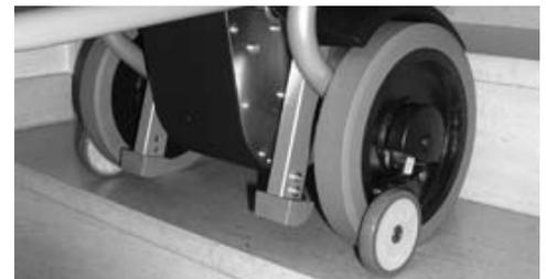
7. Again push the **escalino** all the way to the edge of the step, i.e. until the sensitive rolls of the security brakes stop the **escalino**.
