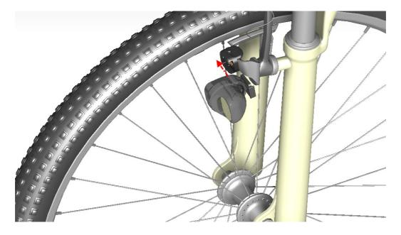
At each Magnic Light unit you find a factory pre-assembled clip for insertion into the click adapter(CA). Now, move the lamp with this clip in the click adapter until you hear a distinct click.
