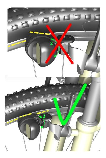
Adjust the clip on the semicircular arc (2) of the lamp holder so that the black nontransparent part of the Magnic Light lighting unit (dashed yellow line) is aligned parallel (horizontically) to the tangent vector to the rim.
