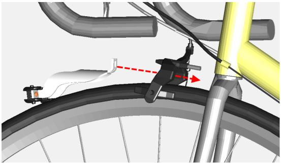
Then move the base adapter A3 according to the drawing through the brake body.
