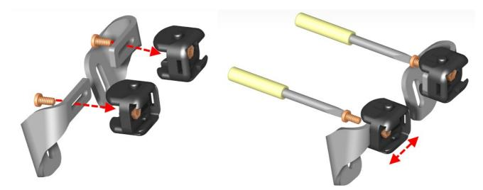
First attach the black click adapters at the corresponding base adapter using the included 4mm bolts S1 and nuts M1. The exact adjustment is done later, so at the moment you should not tighten the screws. Mount the nuts (M1) in front position inside click adapter CA as shown in the picture and not on the back at the aluminium adapter to avoid damage of the click adapter caused by high pressure!
