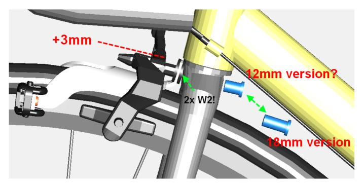
Screw the brake body with additional base adapter firmly. Since the adapter A3 plus the washers W2 have a thickness of 5mm, it may be that your current sleeve nut is not long enough to take to the threads of the brake screw. In this case you need a longer sleeve nut, you get low on our Webshop. Don't tighten the sleeve nut with torque higher than 6 Nm!
