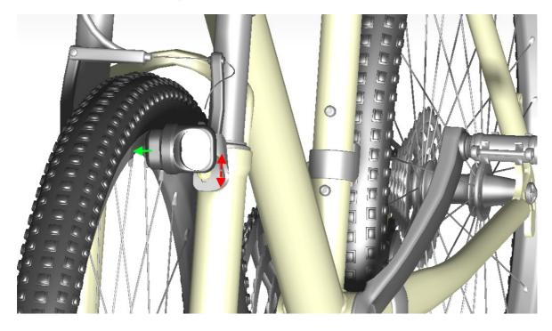
Now set up the base adapter (A1, A2) in height by the screw of for the brake boss(red arrow): The center of the lamp should be slightly below the rim center (green arrow). Even in case of very thick tires at least 3 mm distance to the tires should remain. Tighten the brake bosses screw again firmly according to brake manufacturer's instructions(normally torque: 5-7 Nm).
