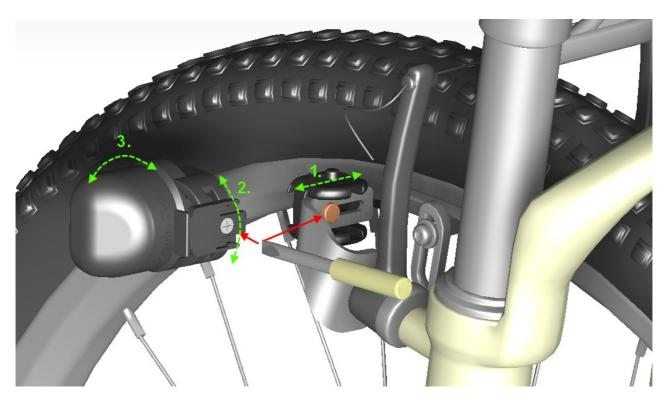
Now adjust the distance of the lamp to the rim by screwing the screw S1 to the click adapter (1). Even for wheels running smoothly at very least this should be 3mm but not to exceed a distance of 9mm. Then tighten the screw S1 with a torque of 1 Nm medium tight. Mount the nuts (M1) in front position inside click adapter CA and not on the back at the aluminium adapter to avoid damage of the click adapter caused by high pressure!
