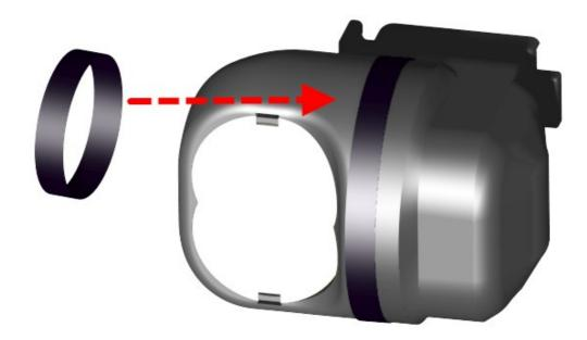
Drag the rubber band so far on the lamp unit, that it covers the edge of rotation between the generator and headlight section entirely. Since the rubber ring has a tight fit on the housing, the water inlet and, in particular, the penetration of dirt is prevented. The rubber ring may remain permanently on the lamp.
