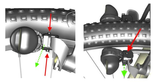
You can remove the lamp unit from the click adapter by simultaneously pressing the two buttons on the adapter firmly and then pulling out the lamp unit from the side of the anchor.
