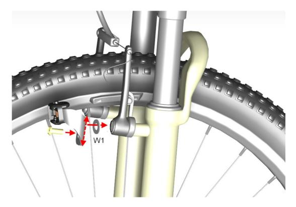
*By the long slot in the base adapter you can do the height alignment of the adapter later to ensure the lamp runs exactly on rim height.*
