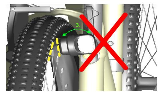
Adjust the clip vertically so that the black non-transparent part of the Magnic Light unit is aligned parallel (dashed yellow lines) to the rim. Note that some rims have a sloping profile (V-profile). In this case, the lamp unit should be set to an angle so that the gap between the rim and light unit has a very uniform width and this way maximum power can be achieved. In the image above, you can expect a significant loss in performance due to the oblique attachment.
