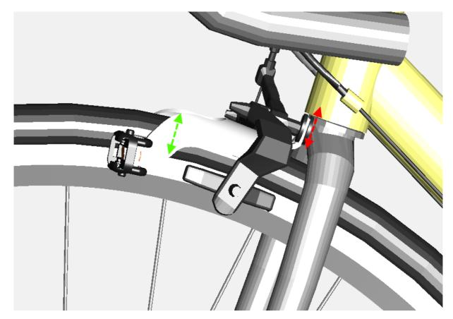
You can easily modify the height and thus the distance from the tire (green arrow) by the slot on the adapter (red double arrow).
