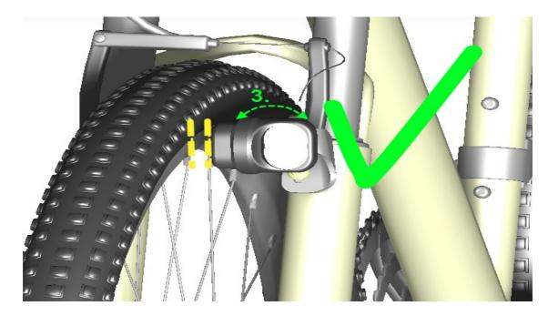
Here it is done right: The dynamo is aligned parallel to the rim profile and thus can operate much more efficiently.
