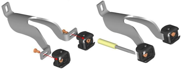
Attach the black click adapter using the included 4mm bolts S1 and associated nuts at the base adapter. The exact adjustment is done later, so you should not tighten the screws at the moment. Mount the nuts (M1) in front position inside click adapter CA and not on the back at the aluminium adapter to avoid damage of the click adapter caused by high pressure !
