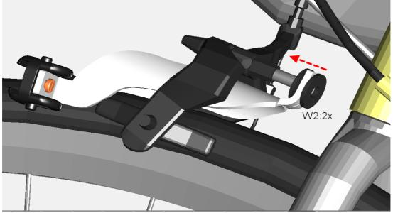
Push the long mounting screw of the brake body through the slot of the adapter. Don't forget to set the washers W2 on both sides of the adapter to prevent damages and breakage of the adapter!
