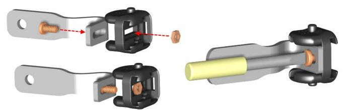
First attach the black click adapter CA using the included 4mm screw S1 and nut M1 at the associated base adapter A4. The exact adjustment is done later, so you should not tighten the screw in the first step. Mount the nuts (M1) in front position inside click adapter CA and not on the back at the aluminium adapter to avoid damage of the click adapter caused by high pressure!
