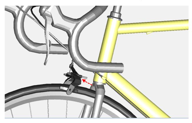
To do this, first remove the sleeve nut that holds the brake body into the fork with an Allen wrench and pull out the brake body forward from the fork.
