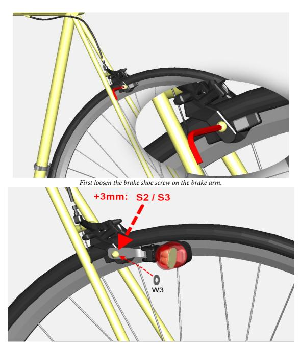
Then screw the brake shoe in addition with with the adapter inferior according to the manufacturer (normally with a torque of 8-9 NM) (as in the picture). The following should be noted: The adapter will also requires 3mm extra length of the screw. If your previously used screw is not long enough, you have to use a longer screw. In your package are two extended screws S2 and S3 in sizes M5 and M6 that are suitable for most rim brakes. Don't forget to underlay the washer W3.
