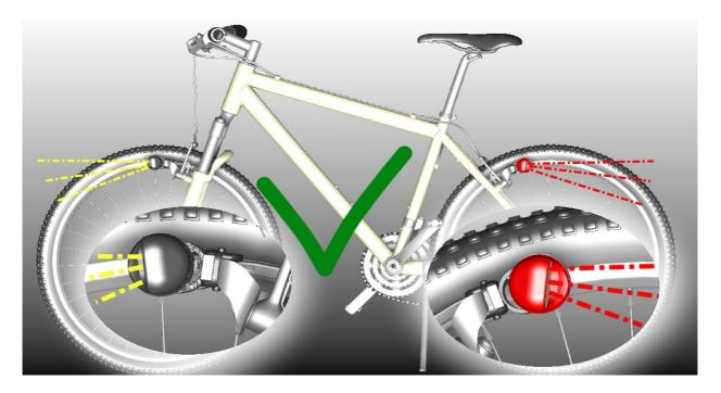
Here, front and rear lights are set correctly: both are aligned below the horizontal and avoid glare. The illumination of the driving range is also better.
