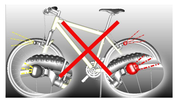
In the picture above the headlights and the rear light are aligned too far to the top. This creates a strong glare and worsens the illumination of the own field of vision.
