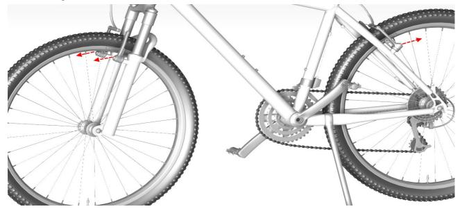
To do this, first remove the brake boss bolts that hold the brake arm and take them off (the red arrows). Now screw the brake bosses screw removed earlier at the base adapter with underlyig washer W1 and initially tighten the screw only loosely.
