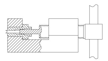
Figure 4-3 Electrode Advancing Tool
