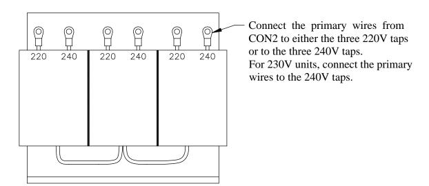
Figure 5-1 220/230/240V 60 Hz Three Phase Transformer
