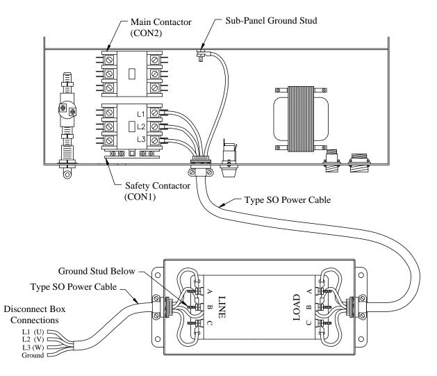
**Figure A-1 Primary Power Connections**
