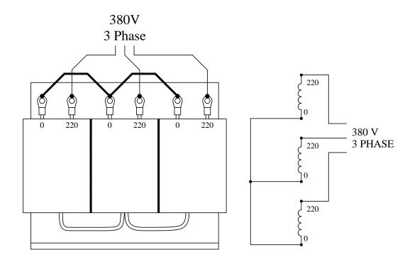
Figure 5-3 380V 50 Hz Three Phase Transformer
