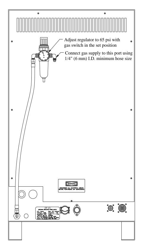
Figure 3-4 Gas Supply Connections
