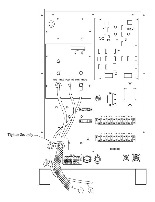
Figure 3-2 Power Supply Output Connections
