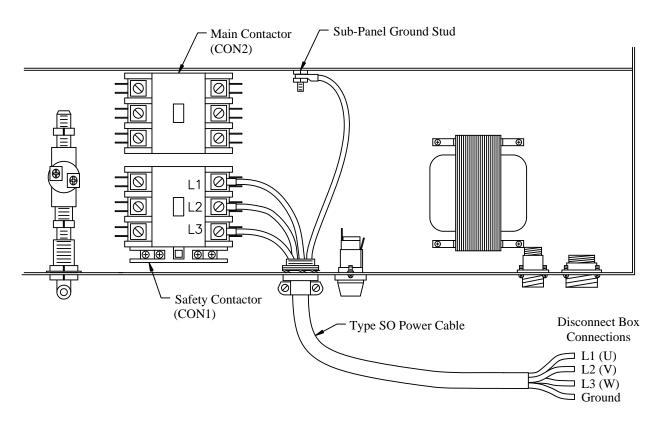
**Figure 3-1 Primary Power Connections**
