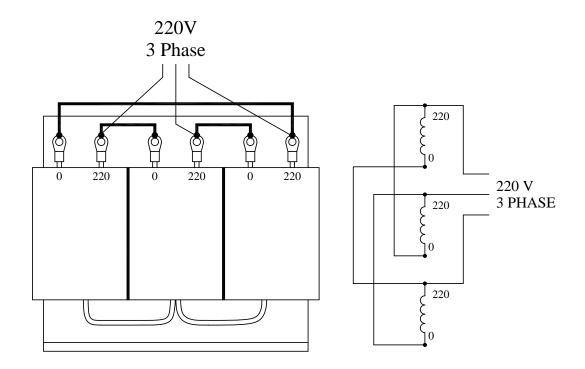
Figure 5-2 220V 50 Hz Three Phase Transformer
