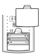
3. Replace the battery compartment door.
