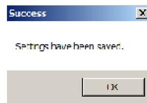
Power down the MetPak Base Station and apply power back to the MetPak Base Station to complete setting changes.
