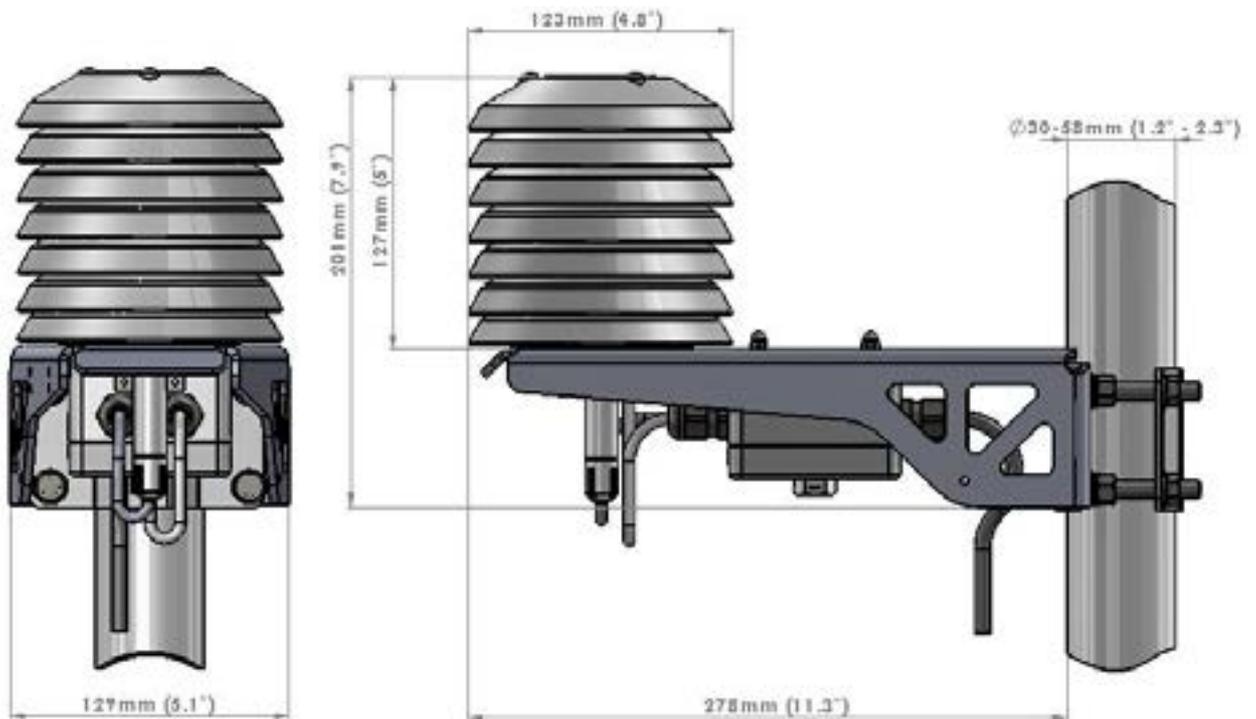
Figure 10 Mounting and Dimensions for MetPak Base Station
