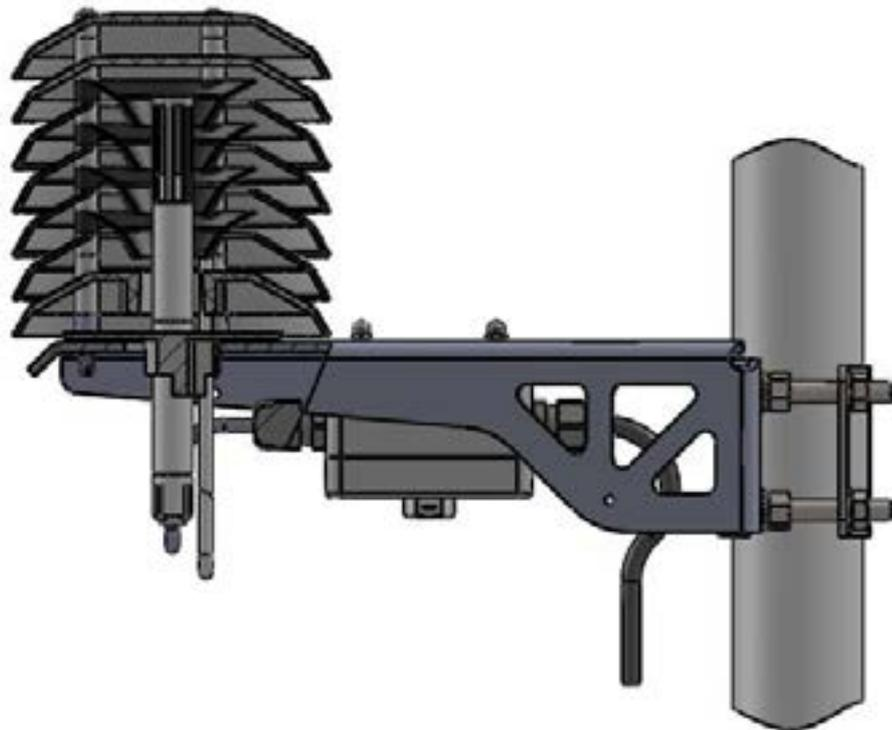
Figure 2 Position of Temperature and Relative Humidity Probe in the Radiation Shield
