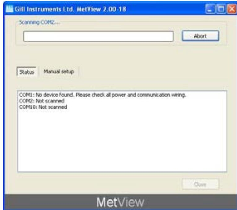
Figure 12 Scanning for MetPak Base Station Devices
