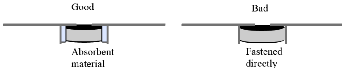
Figure 3.3.4.5 – Microphone Insulating – Recreated with data provided from Veear[42]
