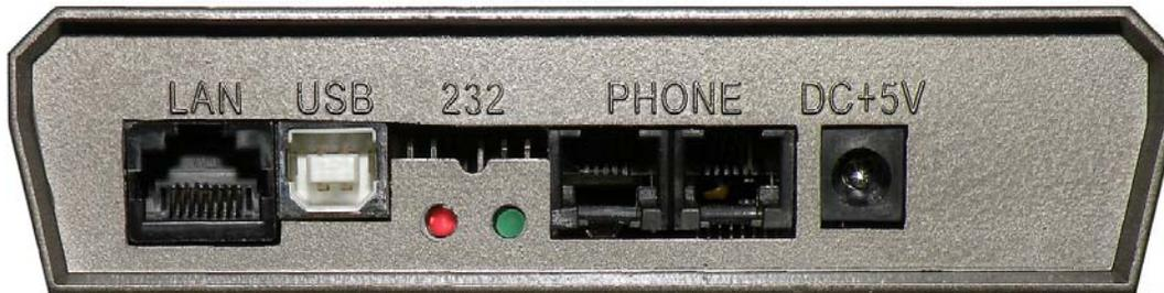
Rear view — RJ-45 LAN jack for connecting to a computer network, USB jack for connecting to a computer via USB, red LED to indicate an active 100Mbps LAN connection, green LED to show LAN activity, two modular phone jacks for connecting to the source of the conversations to be recorded (two channels per jack, image at right), and +5vDC input jack for connecting to power using the supplied AC adapter.
