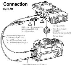
USB cable (accessory of OM-D) To multi-connector terminal
