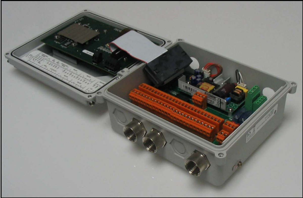
Figure 6: Display Controller Interior
