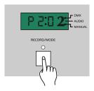
1. Tap the Mode button several times until the a dot LED near Manual lights.
