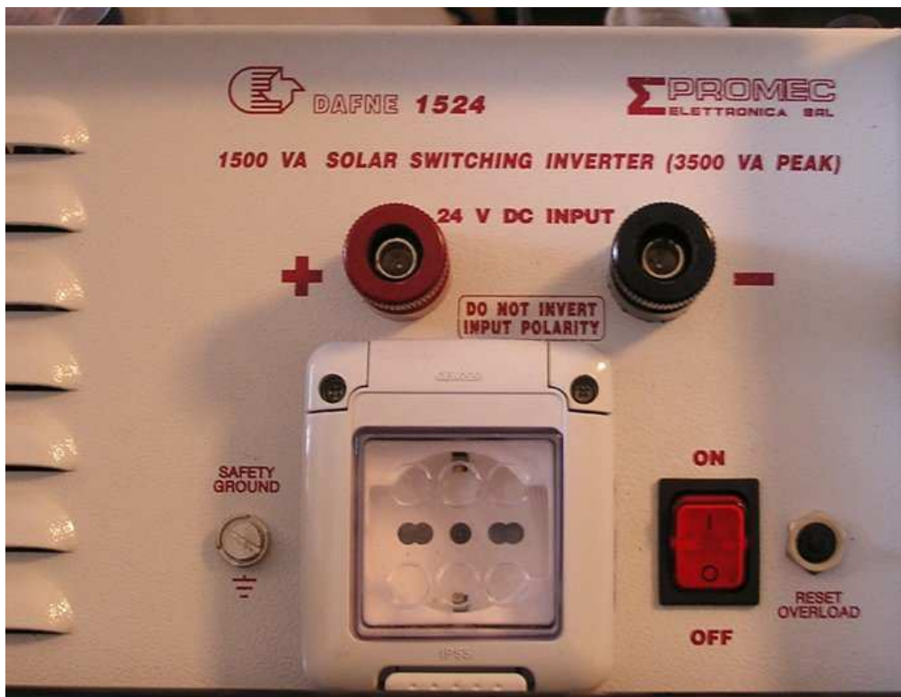
Fig. 5 – The inverter's console with the connections and switches
