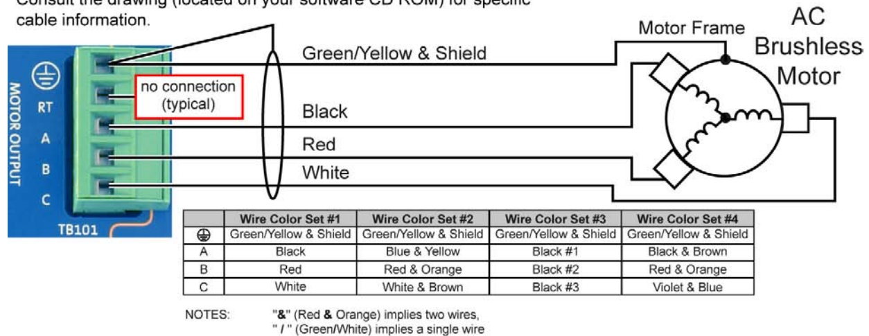
Figure 2-7. Brushless Motor Configuration
