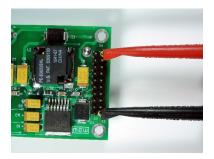
The main battery voltage should be in the range of 8 to 28 Vdc. The power consumed is essentially constant so that higher battery voltage results in lower current draw and vice versa. Rev B and later PWAs are reverse power polarity protected.
