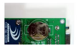
Connect the negative terminal of the battery to J10 pins 1 and/or 2. These two pins are internally connected to each other on the PWB.
